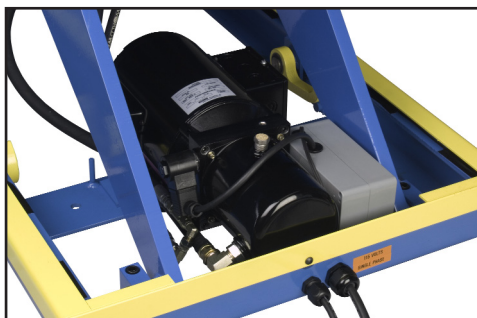
Compact, internal power unit and reservoir combination
